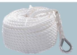
Nylon will stretch by about 20% at 50% of its breakload, compared with 12% stretch for Polyester at equivalent loads.
